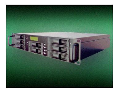
Direct-attached is the easiest way to add storage to your server. Since most servers have a SCSI interface that is underutilized, simply add the RAID 8 to a spare ID on your SCSI chain, and your server's storage capacity is increased many times over.
